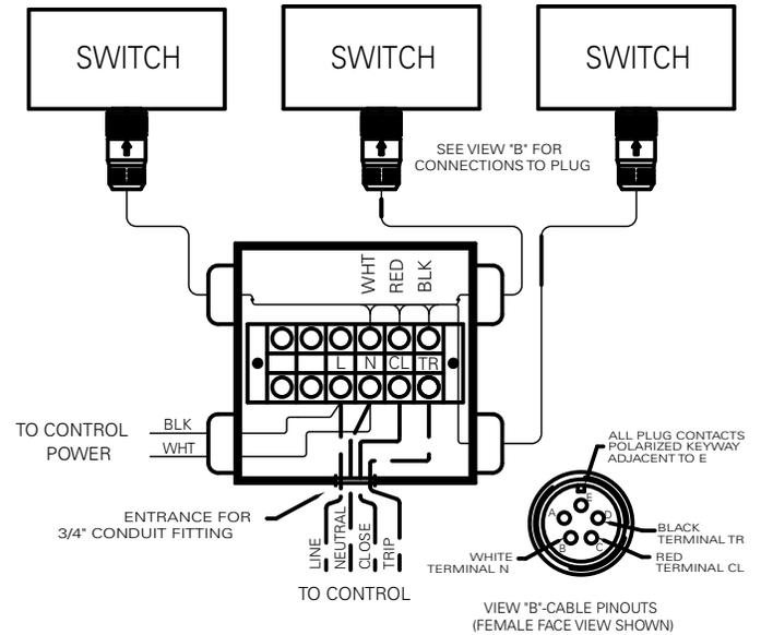
**Figure 4. J-Box switched control connections.**
