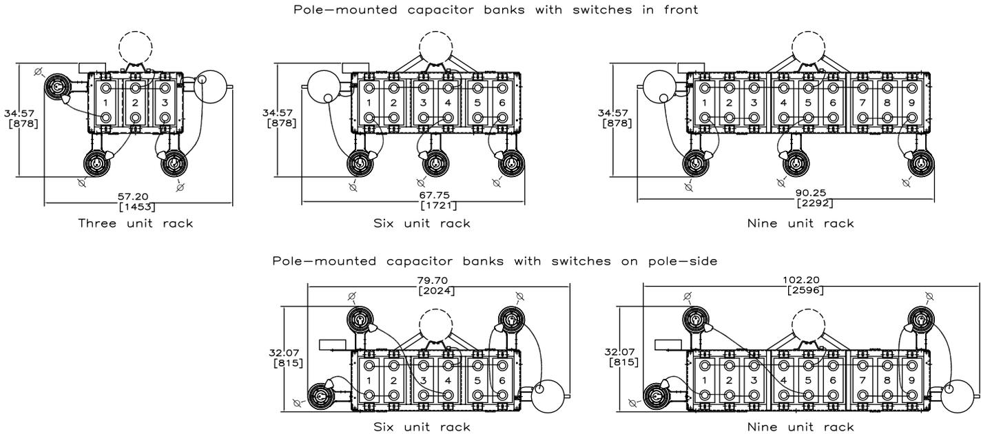
**Figure 5. Capacitor rack assemblies 95 kV BIL with 50, 100, 150, 200, 300, 400, 500, or 600 kvar units**
